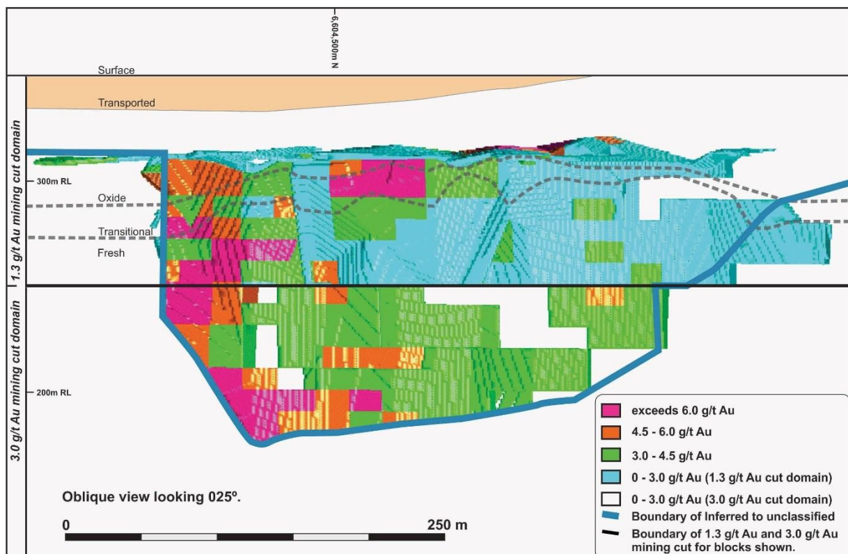
Figure 3: Long section (oblique view looking 025 degrees) of the Gimlet Resource model, depicting grades and cut-off for both open cut and underground mining depths. See text below for more detail.
