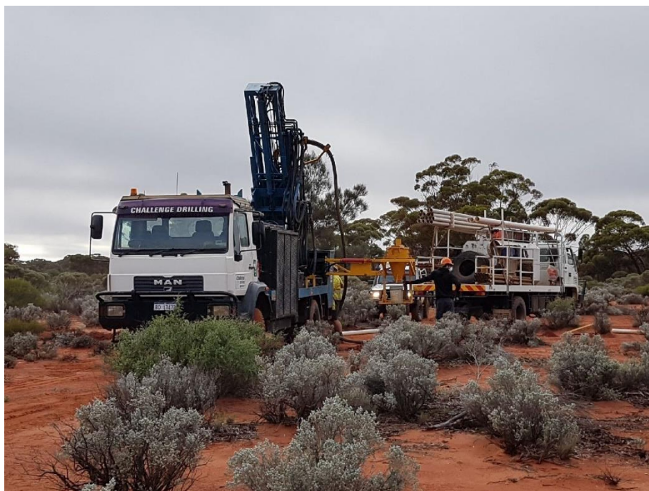
Figure 4: Aircore drilling now underway at Gimlet
