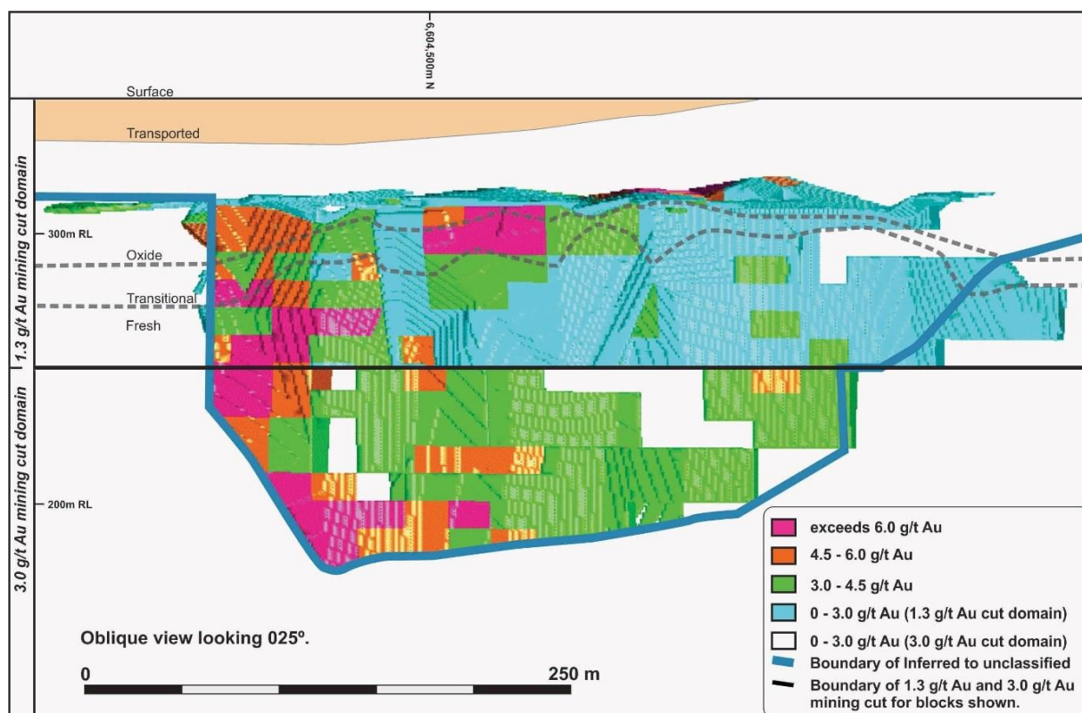
Figure 3: Long section (oblique view looking 025 degrees) of the Gimlet Resource model, depicting grades and cut-off for both open cut and underground mining depths. See text below for more detail.
